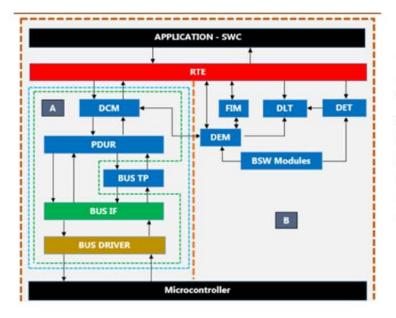
In Application Layer, there are SWCs that are responsible for monitoring various events like Sensor voltage etc. When there is any discrepancy in the specified voltage then the Monitor SWC will use the look up table provided by the CDD (diagnostic data base file ) to find the DTC code and log DTC(Diagnostic Trouble Code) in Non-Volatile Memory Location through DEM(Diagnostic Event manager) Module.
