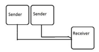
• If the sender-receiver communication configured as non-queued, then the receiver always has access to the last sent data.
